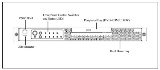
Figure 2 600r CallPilot server - front panel LEDs
